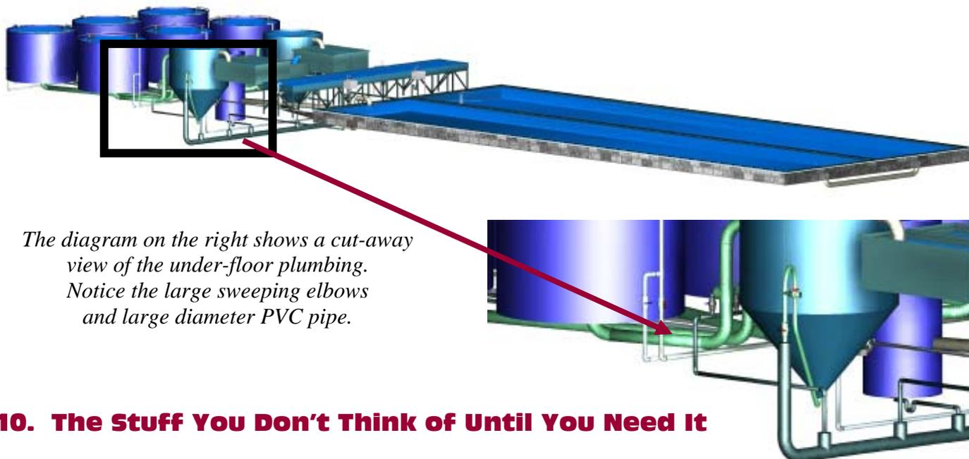
*The diagram on the right shows a cut-away view of the under-floor plumbing. Notice the large sweeping elbows and large diameter PVC pipe.*
