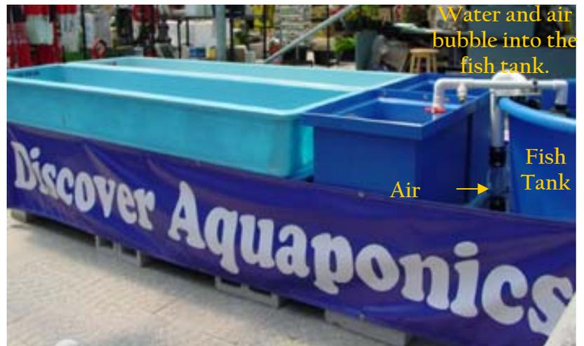
If you are planning your system, I recommend looking into an airlift if you only need to lift the water a small amount. Often, The same airpump will supply air to the airlift, diffusers in the fish tank and an air distribution grid in the grow bed (raft or media filled bed). The increased oxygen levels that you will have as a result of using air to move water will be beneficial for your fish, plants and bacteria and your system will be healthier overall.
